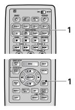
1 Prepare the source you want to record and put the receiver in that function. Set SIGNAL SELECT to DIGITAL.
